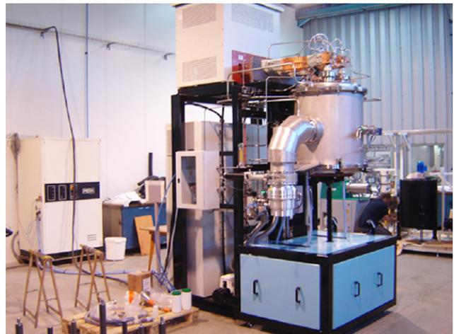
**The CRG-20 oven has a maximum temperature of 2000° C.**
