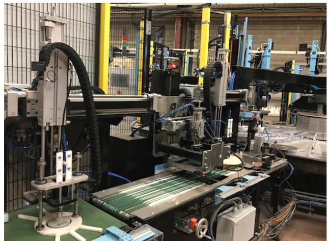
The 8TT320 machine is designed for automatic decorating with ability to process from 4 to 8 colors using silicon pads and screens for flatware and some holloware articles.
