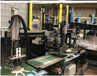
The 8TT320 machine is designed for automatic decorating with ability to process from 4 to 8 colors using silicon pads and screens for flatware and some holloware articles.
